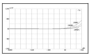
Figure 9. Representative DC Offset vs. Gain
