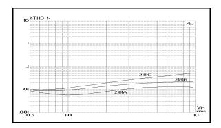
Figure 12. 1 kHz THD+Noise vs. Input Level,-15dB Gain
