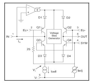
Figure 5. Simplified Internal Circuit Diagram
