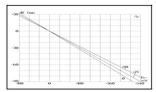
Figure 8. Gain vs. Control Voltage(E<sub>C-</sub>) with Temp (°C)
