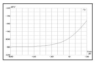
Figure 4. 2181 Series Noise (20kHzNBW) vs. Gain
