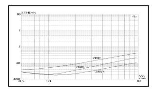
Figure 10. 1 kHz THD+Noise vs. Input Level, 0dB Gair
