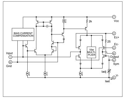
Figure 1. 2181 Series Equivalent Circuit Diagram
