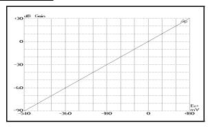
Figure 6. Gain vs. Control Voltage(E<sub>C+</sub>, Pin 2) at 25°C
