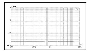
Figure 13. 2181A THD+N vs Frequency, 0dB gain, 1V
