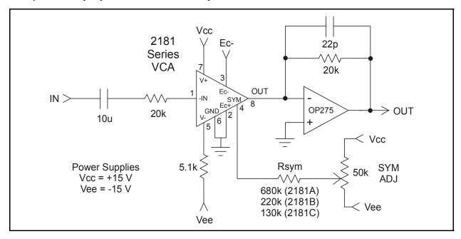
Figure 15. Positive Control Port using Pin 4
