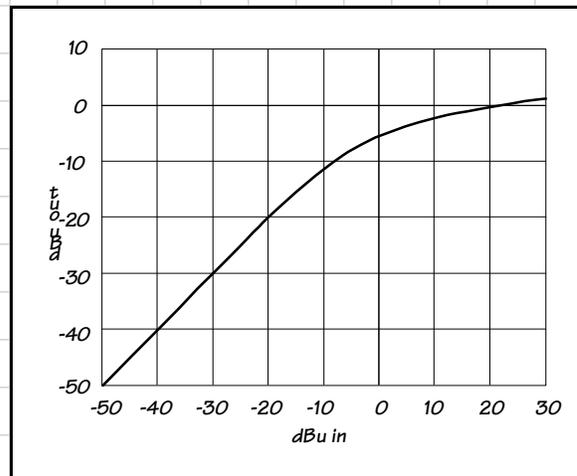
Figure 8. Soft knee threshold characteristic
