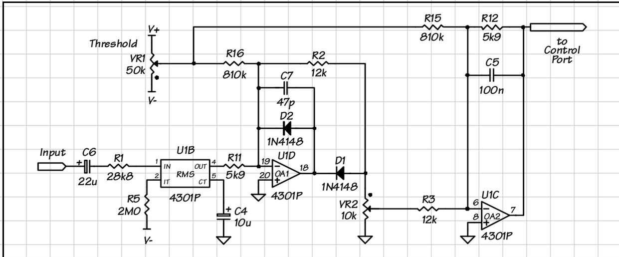
Figure 5. Comp/limiter sidechain with complementary gain and threshold
