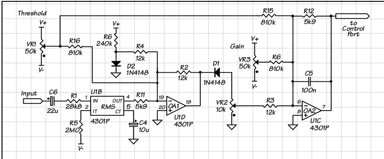
Figure 7. Soft knee comp/limiter with complementary gain and threshold
