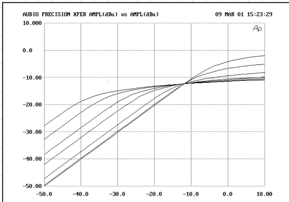
Figure 9. Transfer characteristic of the "One Knob Squeezer"
