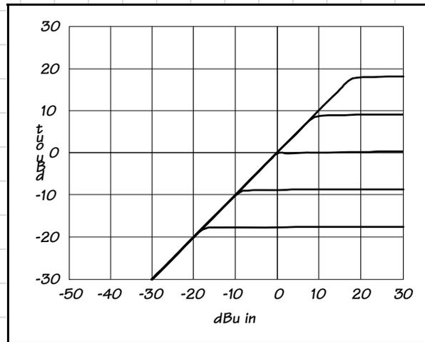
Figure 2. Typical hard knee threshold characteristic
