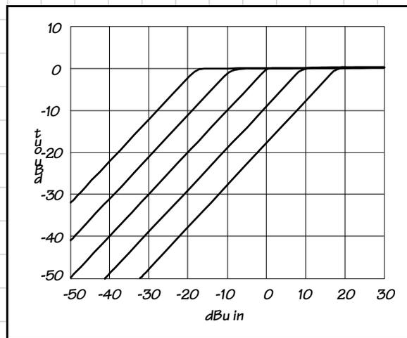
Figure 6. Control characteristic with complementary gain and threshold
