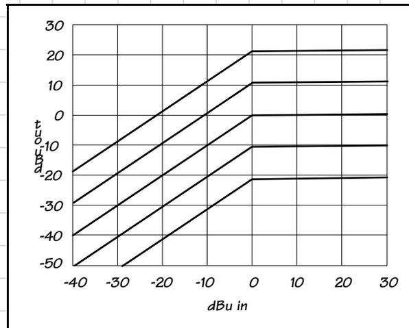
Figure 3. Typical makeup gain characteristic
