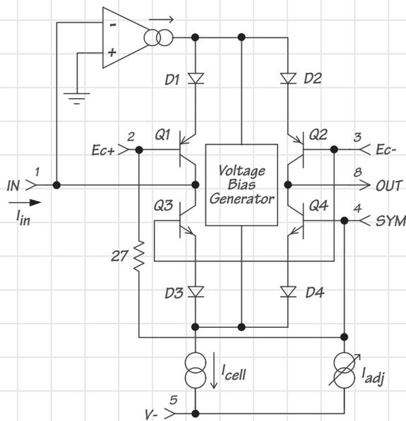
Figure 2: Simplified Internal Circuit Diagram
