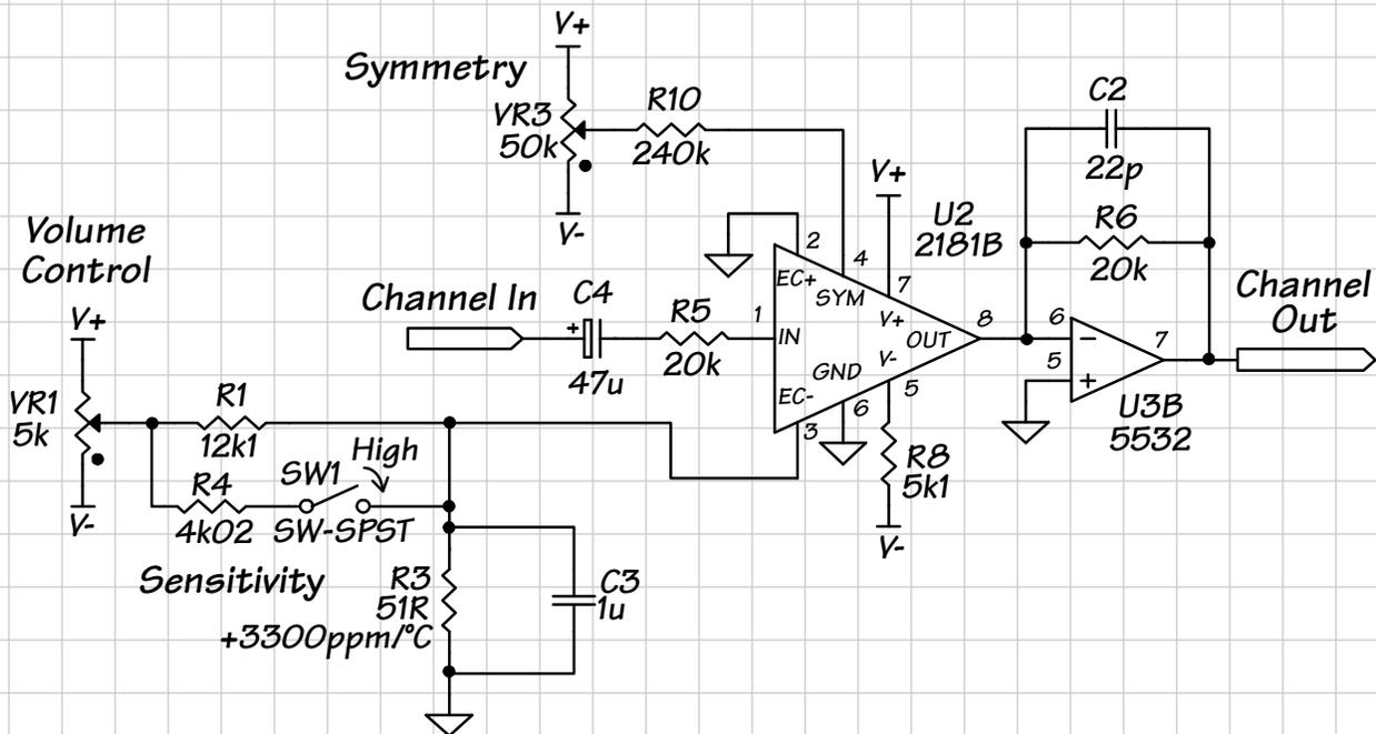
Figure 4. Volume control with switch selectable sensitivity
