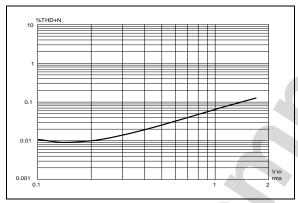
Figure 5. VCA 1kHz THD+Noise vs. Input, +15 dB Gain
