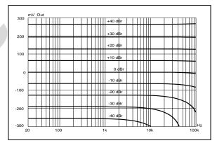
Figure 10. Detector Output vs. Frequency at Various Levels
