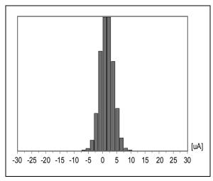
Figure 13. Representative  $R_{\mbox{\scriptsize G}}$  Input Bias Current Distribution
