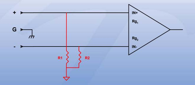
Must provide a DC current path to supply the amplifier input bias current
