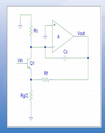
$$\frac{R_{C} \cdot A}{V_{in}} = \frac{\left[r_{e} + (R_{F} \| R_{G}/2)\right] (R_{C}C_{M}S + 1)}{R_{C} \cdot A} \cdot \frac{R_{G}}{R_{F}} = \frac{A}{1 + A\beta}$$
