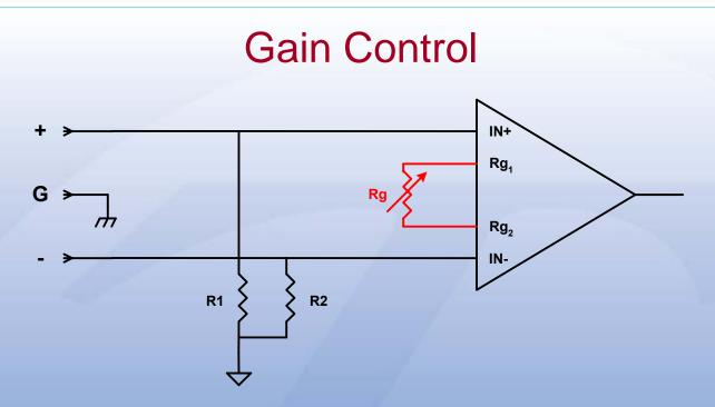
The amplifier is often designed to vary gain using a single variable resistor ( $R_{\alpha}$ )
